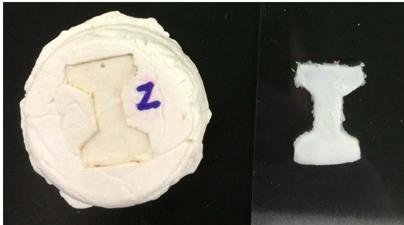
Figure 3.2 One of plaster molds and dog bone specimens
