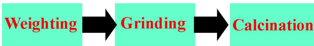
Figure 3-2 Schematic of synthesis process for solid state reaction method.
