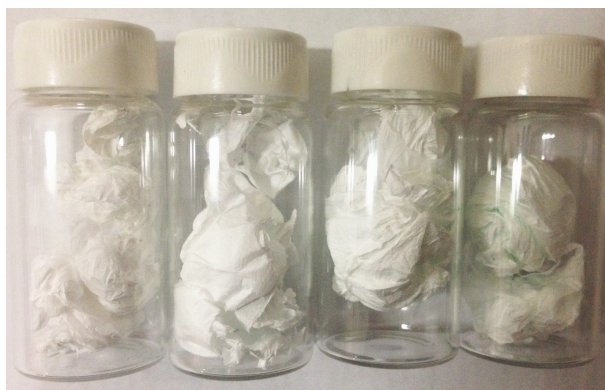
Figure 10 Eletrospun fibers of (a) PVP; (b) PVP/Cu 2+ (I); (c) PVP/Cu 2+ (II); (d) PVP/Cu 2+ (III)
