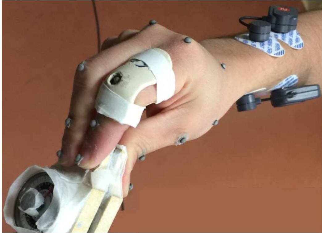
Figure 5.1: Thumb, index, and middle fingers postures with 4 mm markers attached, the PIP joint splinted, and wireless EMG sensors attached to the forearm during chuck pinch performance.
