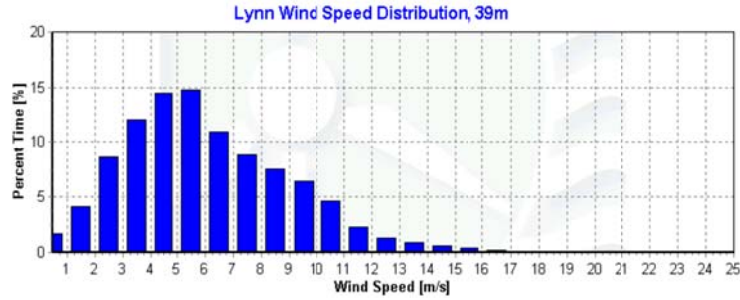
Figure 4.4 A typical wind speed distribution in a period of three months measured in Boston area (RERL Wind Data).
