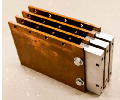
Figure 6.28 Copper plate of the eddy current damper.
