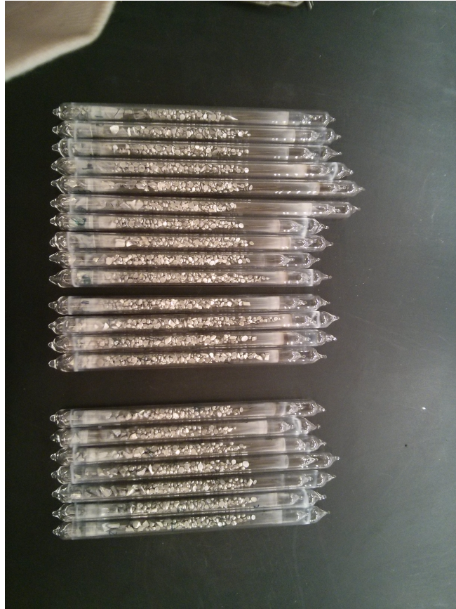
Figure 1: Photo of pieces of Pb, Sn, In, and Te sealed in double layers of fused quartz glass ampoules for the synthesis of \text{Pb}_{1-x-y}\text{Sn}_x\text{In}_y\text{Te} and related materials, to explore potential topological insulator and superconductor properties.
