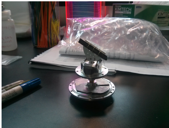
Figure 4: Photo of the \text{La}_{1.9}\text{Ca}_{1.1}\text{Cu}_2\text{O}_{6+\delta} crystal used for the neutron scattering experiments in Section 5. This crystal was obtained from the rod shown in Fig. 3. It is mounted on a goniometer, parts of which are wrapped in cadmium to absorb neutrons and reduce the background due to unintended scattering from the goniometer.
