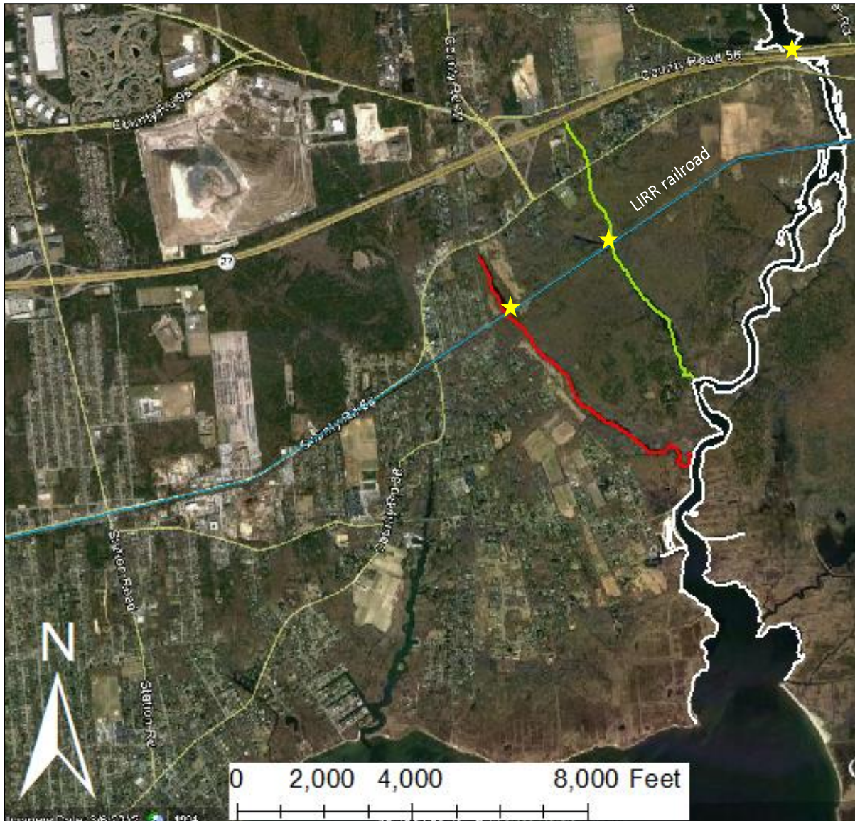
Figure 3.9: Little Neck Run (red), Yaphank Creek (green), and Carmans Rivers (white). The yellow stars show the approximate locations of flow measurements made by Wexler (1988a).
