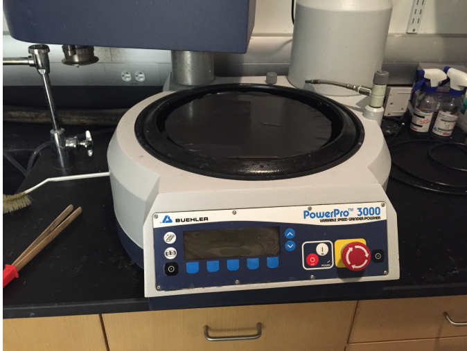
Fig 2.2 Buehler machine used for grinding of samples under constant water irrigation
