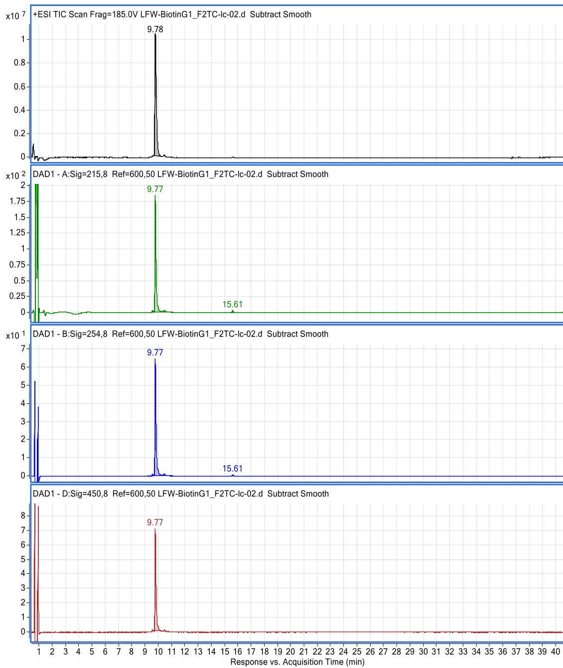
ESI + , TIC (m/z=100-3200) chromatogram for Biotin-G1-FITC DAD1-A, UV=215nm chromatogram for Biotin-G1-FITC DAD1-B, UV=254nm chromatogram for Biotin-G1-FITC DAD1-D, UV=450nm chromatogram for Biotin-G1-FITC Figure 3.36 LC-MS spectrum of biotin-G1-FITC conjugate 3-20
