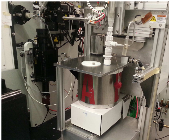
Figure 15: Automounter at the X6A protein crystallography beamline. The automounter's dewar is capable of housing four pucks, meaning it can hold up to 64 samples.
