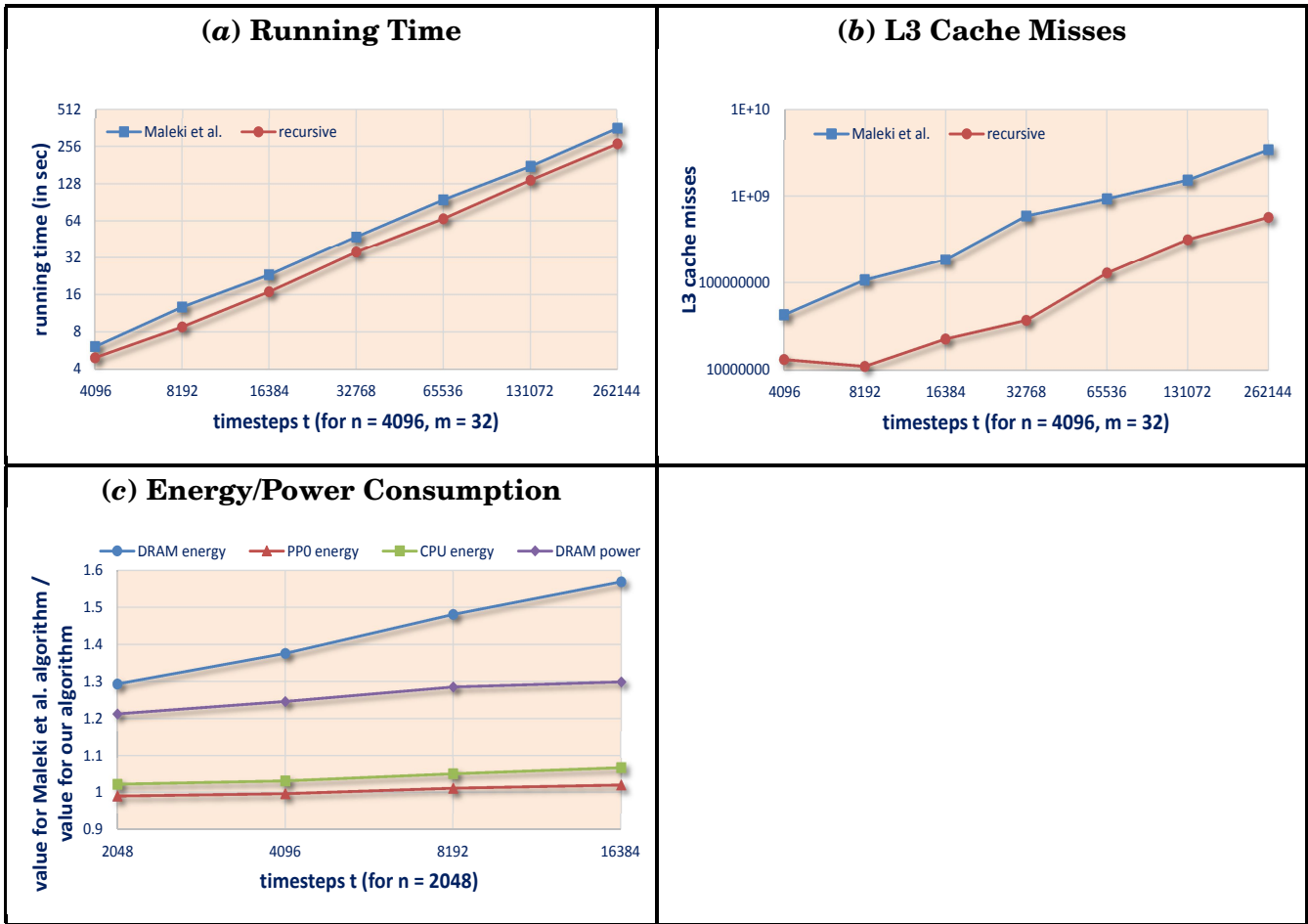
Figure 4.13: Running time, L3 miss and energy/power consumption of our cache-efficient Viterbi algorithm along with the existing algorithms.
