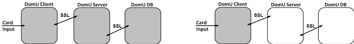
Figure 3.7 osCommerce Card Data Flow (machines found to participate in the card data flow are shown in grey) (left) using vCardTrek; (right) using a packet sniffer.
