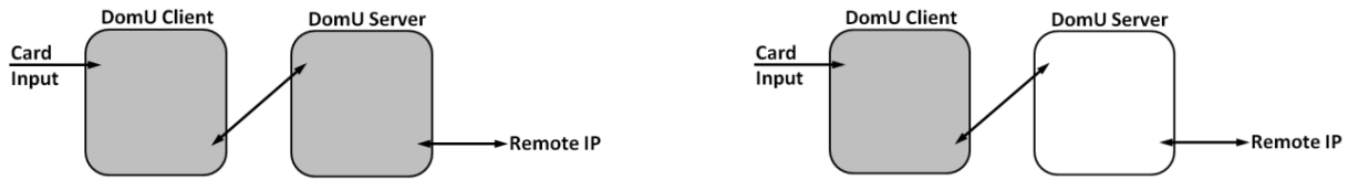
Figure 3.8 CreditLine Card Data Flow (machines found to participate in the card data flow are shown in grey) (left) using vCardTrek; (right) using a packet sniffer.
