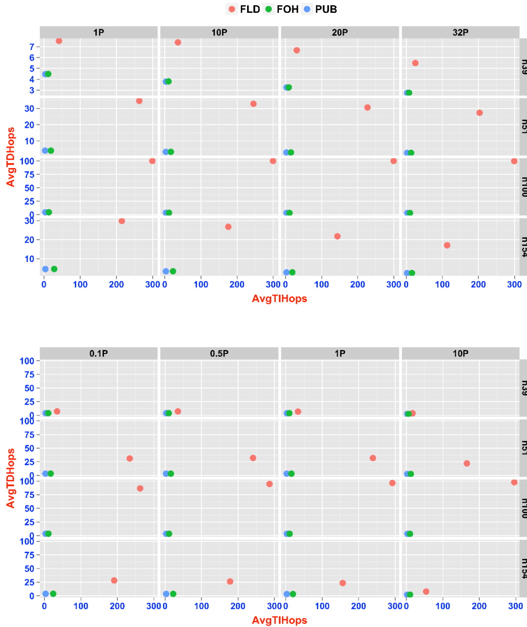
Figure 4-8. Bandwidth costs of CCN-Flooding (FLD - red), CCN-FOH (FOH - green), and CCN-Publication (PUB - blue) for: (a) Cache-Unfriendly Workload (top); (b) Cache-Friendly Workload (bottom)
