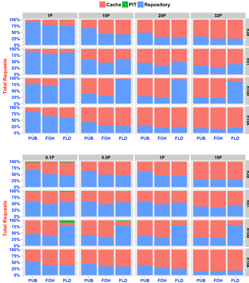
Figure 4-9. Requests satisfied outside the requesting node between Caches, PIT, and Repository for: (a) Cache-Unfriendly Workload ( top ); (b) Cache-Friendly Workload ( bottom )
