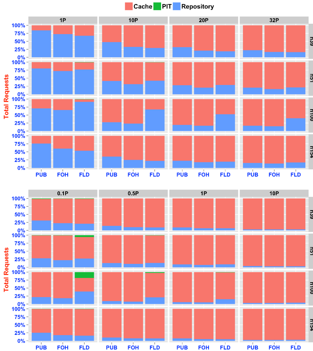
Figure 4-5. Requests satisfied between Caches, PIT, and Repository for: (a) Cache-Unfriendly Workload (top); (b) Cache-Friendly Workload (bottom)
