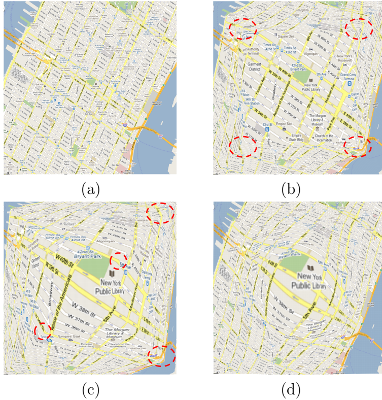
Figure 3.10: Magnification results using different lenses for the NYC street map. (a) Original NYC map. Magnification results using (b) the bifocal lens, (c) the fisheye lens, and (d) the conformal magnifier. The red circles highlight the seriously distorted areas.
