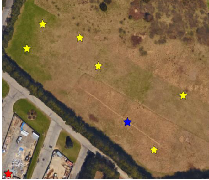
Figure 7.5: Network topology. The blue star refers to the original location of MDC; the yellow stars refer to the location of anchors; the red star refers to the locations of the origin of coordinate system.
