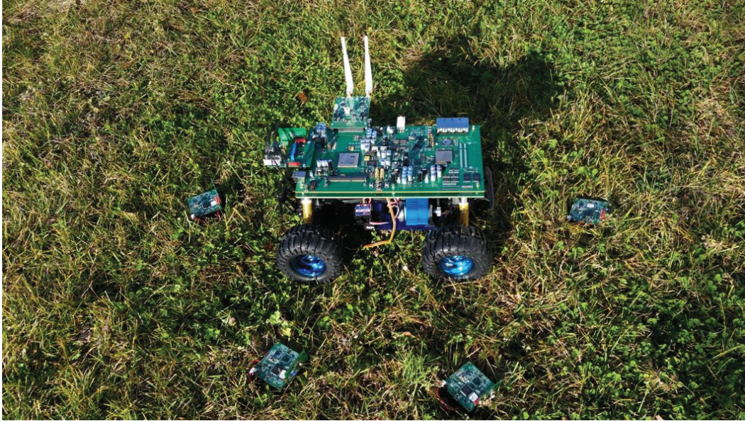
Figure 6.1: A photo of the platform showing 4 wireless sensor nodes and an MDC built with a high performance computing subsystem mounted on a vehicle.
