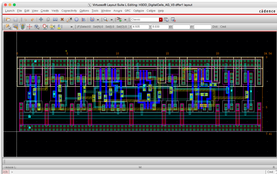
FIGURE 4.4: Layout- D Flip Flop (set/reset) - TSMC 130nm
