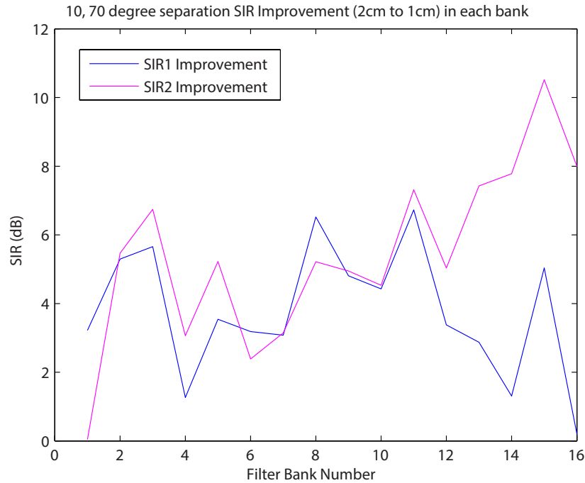
Figure 3.14: SIR improvement of 2cm over 1cm sensor array across all filter banks when there is only noise (SNR=40dB).
