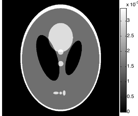
Figure 5.1. A modified Shepp-Logan phantom with display window [0, 0.0034] \text{mm}^{-1} .
