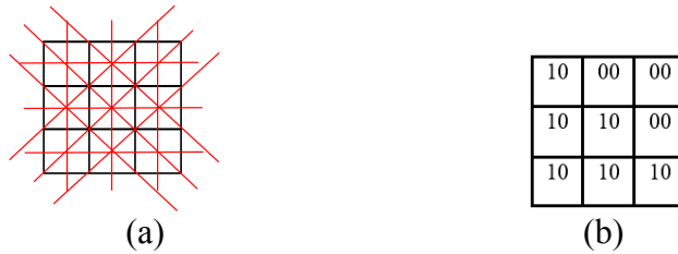
Figure A.1. (a) simulation problem projection geometry, (b) non-uniform phantom; the first elements in each pair indicates the coefficients of cortical bone and second elements indicates the coefficients of water
