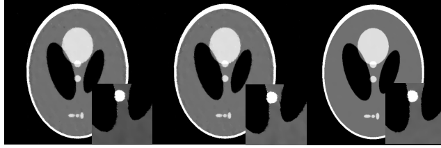
Figure 6.4. The images reconstructed by FBP (1st row), ASD-POCS (2nd row), AwTV-POCS (3rd row) and TVS-POCS (4th row) algorithms from 20 (left column), 40 (middle column), and 60 (right column) projection views in noisy cases, respectively. The display window is [0, 0.0034] \text{ mm}^{-1} for the full FOV images and is [0.0013, 0.0018] \text{ mm}^{-1} for the ROI images.
