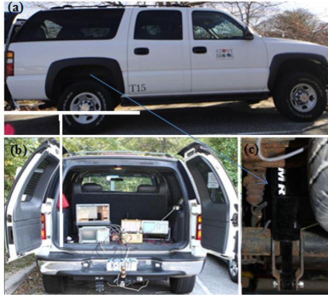
Figure 4 Kinetic energy harvesting device tested on a vehicle [6]
