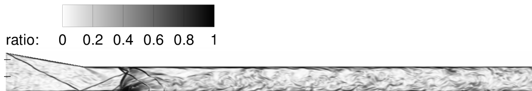
Figure 5.4: The ratio of modeled to total turbulent kinetic energy in the combustion chamber
