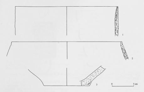
6.5 Slab construction of B.1-B.4 ceramics. 1, ANM 5; 2, ANK 3; 3, ANK 3.
