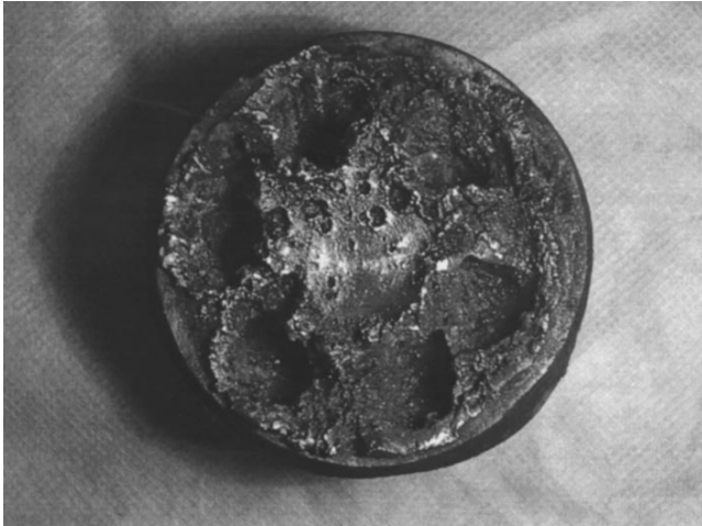
Fig. 4. Craters produced in a steel target by fingers formed on an accelerated plate.
