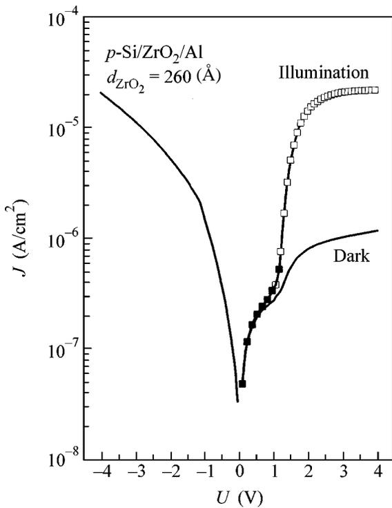
**Fig. 1.** Current–voltage characteristics of the *p*-Si/ZrO<sub>2</sub>/Al structure obtained (solid lines) in the depletion and enhancement modes and (points) in the depletion mode with illumination.
