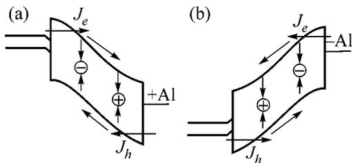
Fig. 4. Schematic diagram of current passage in the Si/ZrO<sub>2</sub>/Al structure for (a) positive and (b) negative potentials on the metal. It is assumed that the generation rate of minority carriers in the depletion mode exceeds the rate of their injection into the dielectric.
