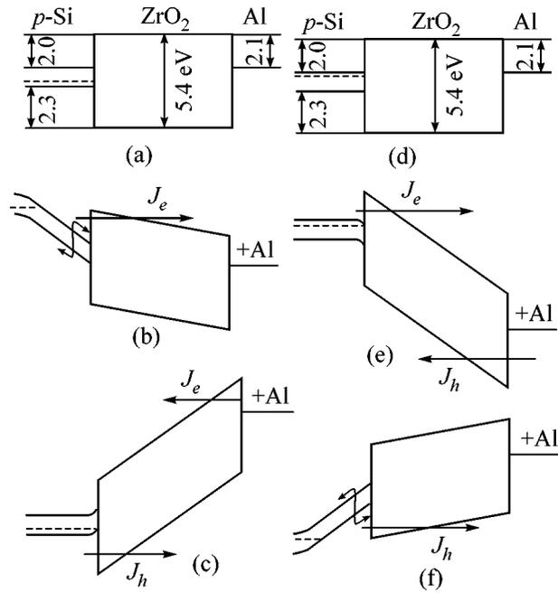
**Fig. 2.** Energy diagrams of [(a), (b), and (c)] *p*-Si/ZrO<sub>2</sub>/Al and [(d), (e), and (f)] *n*-Si/ZrO<sub>2</sub>/Al structures [(a) and (d)] with no applied voltage, [(b) and (e)] in the depletion mode, and [(c) and (f)] in the enhancement mode.
