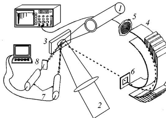
Fig. 1. Experimental setup: (1) femtosecond laser beam, (2) nanosecond laser beam, (3) target, (4) electrostatic mass spectrometer, (5) microchannel plate, (6) aperture, (7) x-ray detectors, and (8) x-ray filters.
