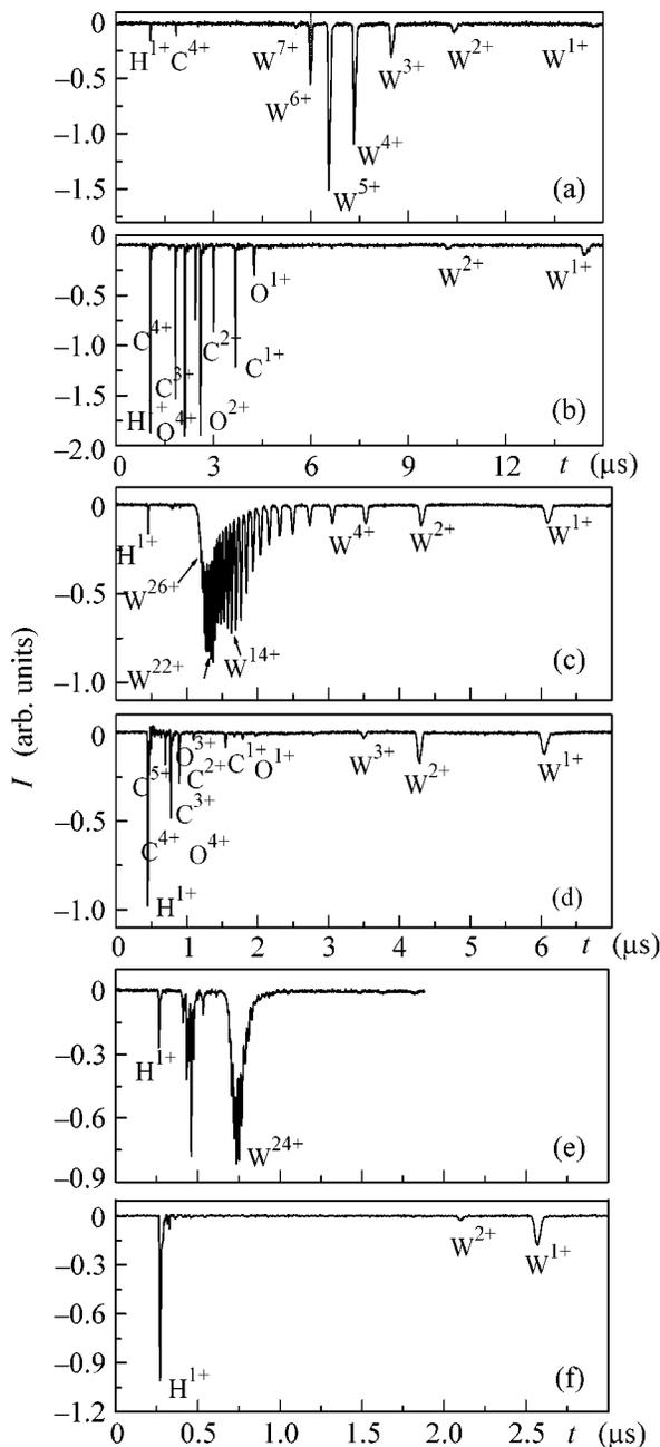
**Fig. 2.** Ion plasma currents from the [(a), (c), and (e)] cleaned and [(b), (d), and (f)] uncleaned tungsten targets for various ion energies per unit charge: (a) and (b) 1.8 keV, (c) and (d) 10.1 keV, and (e) and (f) 28 keV.
