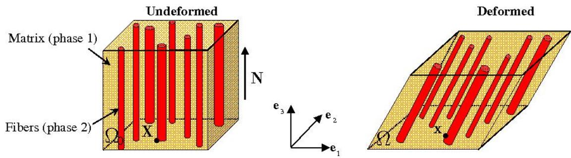
Figure 1: Schematic illustrating a fiber-reinforced elastomer in the undeformed ( $\Omega_0$ ) and deformed ( $\Omega$ ) configurations. Note that, for convenience, the initial orientation of the fibers  $\mathbf{N}$  has been aligned with the coordinate basis vector  $\mathbf{e}_3$ .
