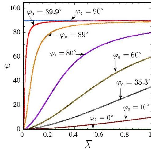
Figure 4: Angle of rotation of the fibers  $\varphi$  (given by expression (43)) in fiber-reinforced Neo-Hookean elastomers subjected to axisymmetric compression (38) for various initial fiber orientations  $\varphi_0$ , as a function of the applied macroscopic stretch  $\bar{\lambda}$ . Note that the results are completely independent of the constitutive behavior of the matrix and fibers, as well as of the volume fraction of fibers.
