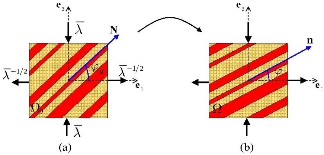
Figure 3: Pictorial representation of the applied loading conditions (38), and the resulting evolution of the orientation of the fibers, as determined by relations (42) and (43).
