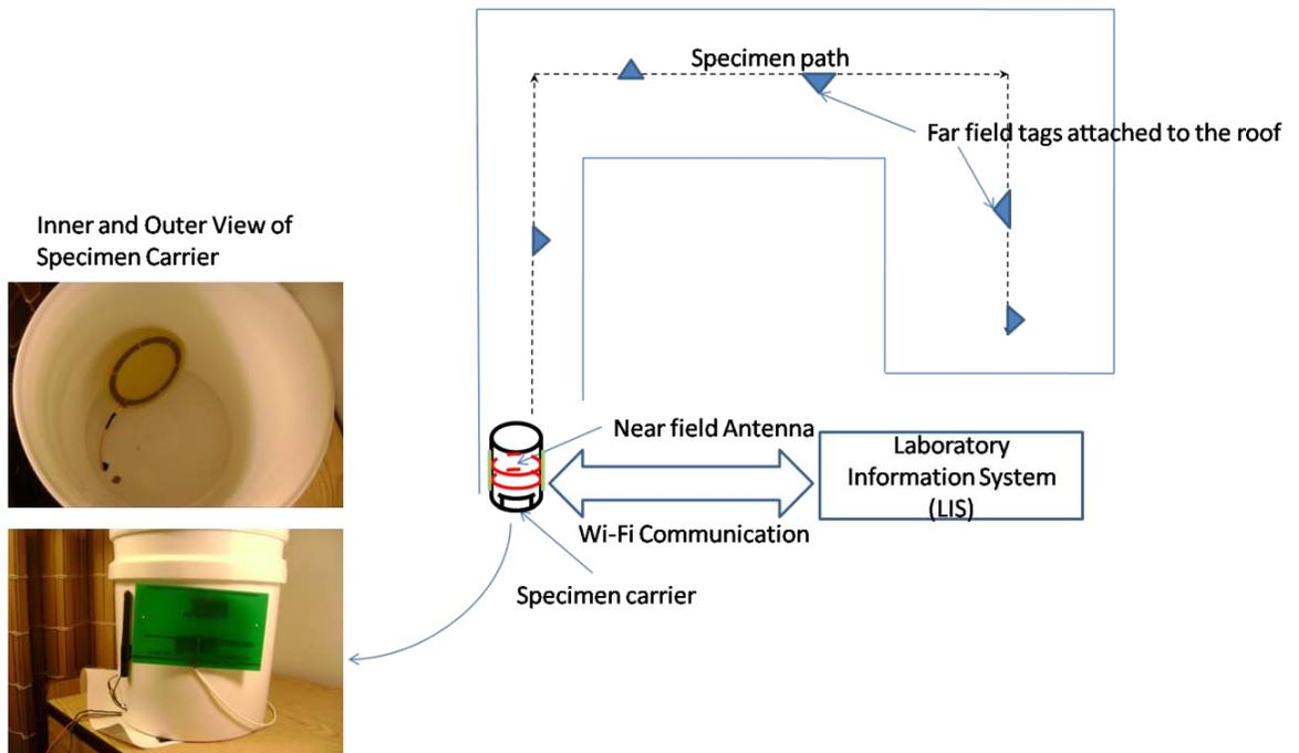
Figure 4.14 Deployment of the system in the hospital
