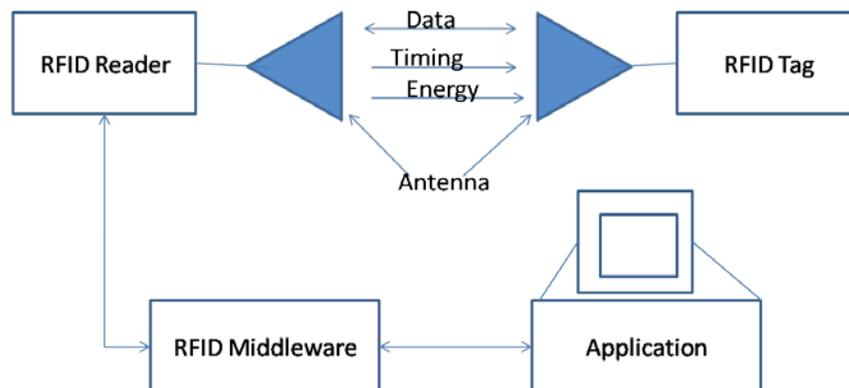
Figure 3.1 Typical RFID System Components.
