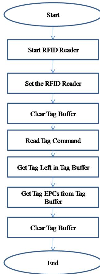
Figure 4.11 Flowchart representing sequence of steps to read a RFID tag
