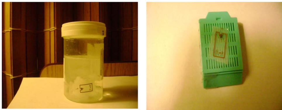
Figure 4.9 Specimen containers with Monza 3 passive RFID tag
