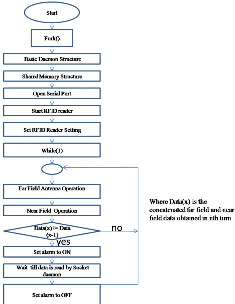
Figure 4.10 Flowchart representing the sequence of operation performed in RFID daemon
