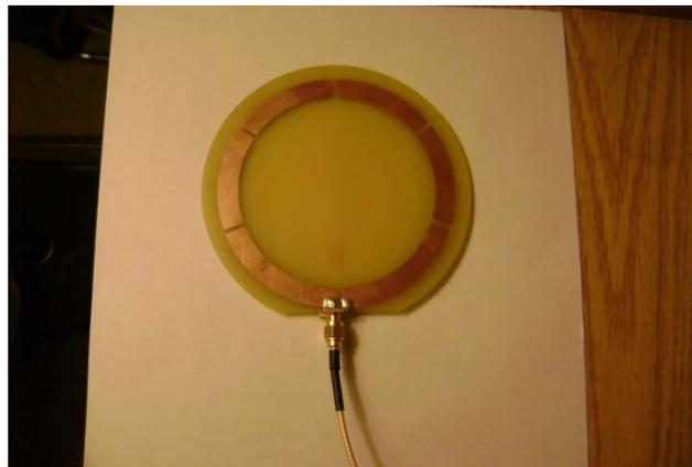
Figure 4.6 Near Field Antenna
