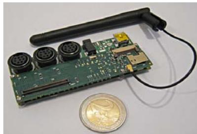
Figure 4.4 Gumstix Verdex-Pro compared with size of a quarter coin
