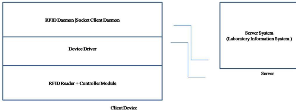
Figure 4.1 Architecture which shows components in the system
