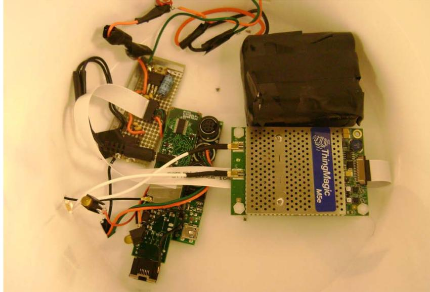
Figure 4.3 Hardware Assembly of Specimen Carrier placed inside the bucket
